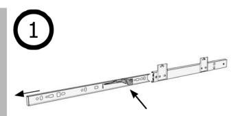
Open one of the runners **b** fully apart by pressing up or down on the grey lever.
