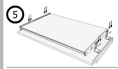
Screw down the brackets **e** to the underside of a shelf, using wood screws **c** ensuring the edges are lined up correctly.
