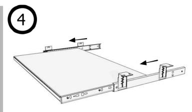
Slide both sections of the runners **b** back together again as shown.
